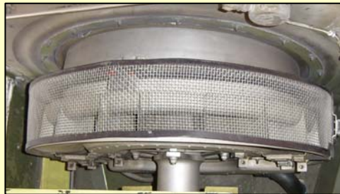
Inertial Particle Separator With Pleated Screen
